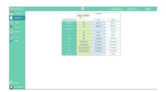
Solaris controlling software offers a simply laid out, yet powerful platform for experimental design planning and process control. The graphical user interface enables the intuitive selection and adjustment of control functions.
