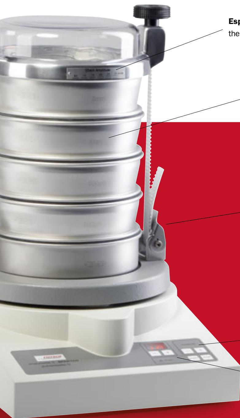
**Especially practical** Optical display of the amplitude during sieving.
