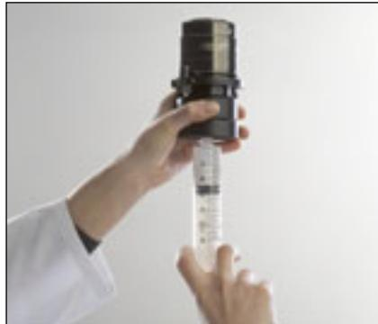
After grinding in suspension the FRITSCH Special Emptying Device with 2 sieves enables a quick and easy separation of the grinding balls and suspension. For this purpose, the device is firmly attached onto the grinding bowl, the suspension is drawn out with the syringe and the balls remain in the bowl.
