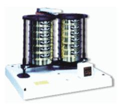
Ro-Tap® RX-94 Test Sieve Shaker utilises the same traditional design as the RX-29 and RX-30 models. In addition, the unit features a cavity that allows for two "stacks" of 8" diameter test sieves. This allows for twice the processing capacity in nominally the same time required to complete one test.
