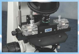
The CELL contains 4 electrodes fitted into perfectly symmetrical chambers - Easy to use & to clean
