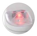
Red Error or emergency stopped, or initializing during power on
