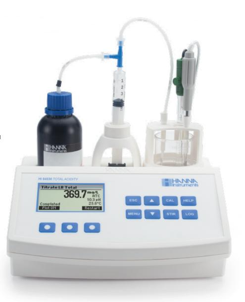
This mini titrator includes a pre-programmed analysis method based on the Standard Methods of Water and Wastewater Determination. It uses a powerful algorithm which analyzes the shape of the electrode response in order to determine when the titration reaction has reached completion.
